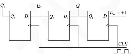
If  $Q_1$ ,  $Q_2$  and  $Q_3$  are set to zero initially, then the output after the arrival of the second falling clock (CLK) edge is
