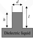
The plates of the capacitor are kept at a constant voltage difference V. Ignoring effects of surface tension, the height h upto which the liquid level rises inside the capacitor, is
